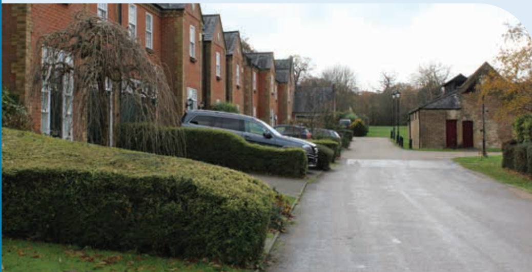
Image 6.18: On plot frontage parking that does not dominate the street scene and provides space for softening vegetation.
